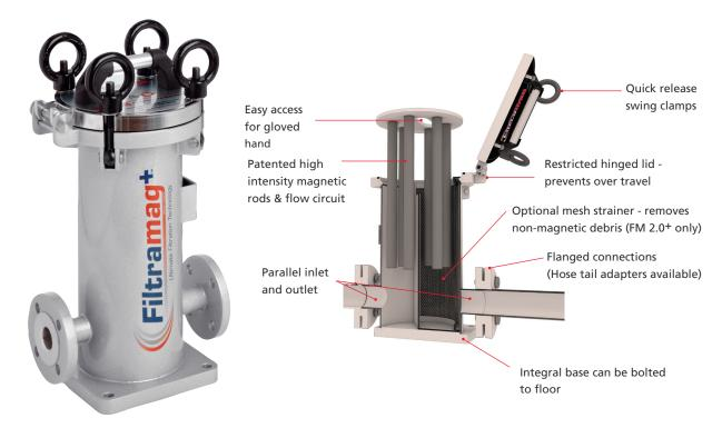
Robust high performance magnetic filter with Dual Flow Technology to maximize collection capability. Easy installation with operation up to 290 psi (20 bar).
