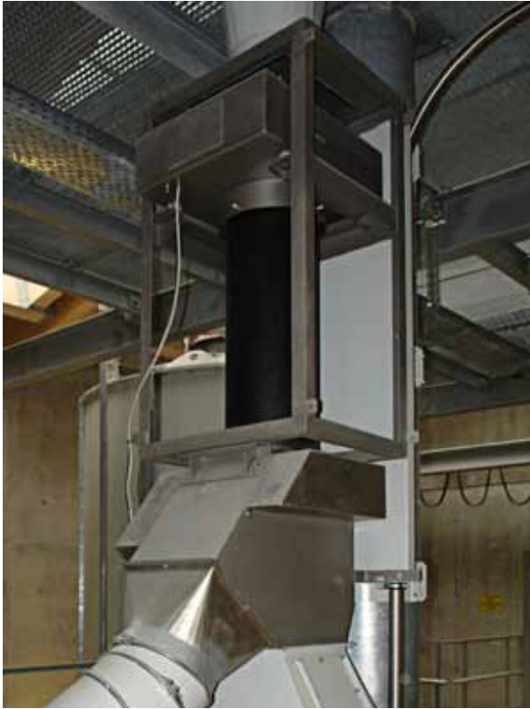
Metal separator GFR DUAL used for machinery protection during wood pellet production
