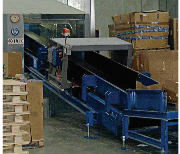
Tunnel metal detector DLS analysing recycling material before the granulator
