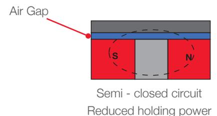
As the air gap increases the magnetic performance reduces.
