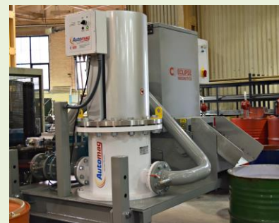
OSL cutting Technology Magnetic Filtration
