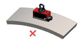
Magnet across increases clamping at possible point of peel.
