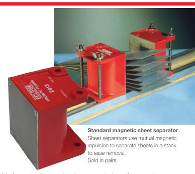
It's important to order the correct size of separator for the size of material to be separated. If the items are half the width of the separator the top items can flip onto the face of the separator instead of being separated.
