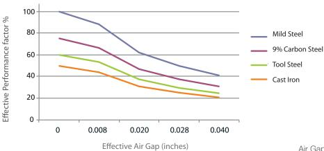
As the air gap increases the magnetic performance reduces.
