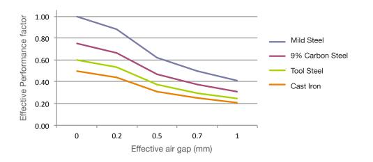
As the air gap increases the magnetic performance reduces.
