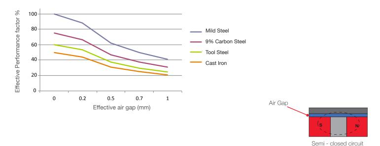
As the air gap increases the magnetic performance reduces.
