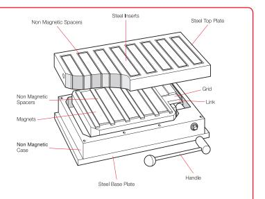
d off by moving the central magnet pack **A**. When it magnetism is directed into the workpiece, when it ate magnetism is directed away from the workpiece.
