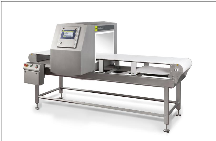
VARICON+ metal detection system with C-SCAN GHF detection coil to analyse bags or E2-boxes.
